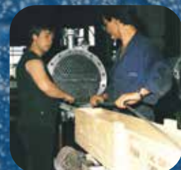
Ethylene glycol exchangers. Courtesy: Bronswerk Heat Transfer, Netherlands
