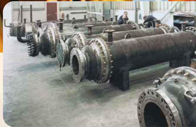
Heating crude oil with hot jacket water from pumping stations Crude oil pipeline
