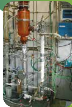
Thermosyphon reboiler studies. University of Braunschweig
