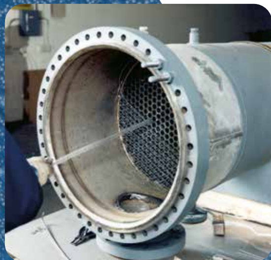
'Key Link' system being fitted to citric acid heater. Courtesy: Milles Laboratories, USA.
